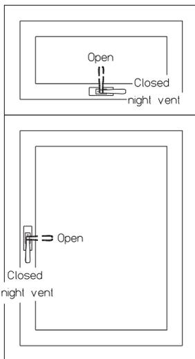
Push button on handle (if applicable) rotate handle 90 degrees and push window open.
