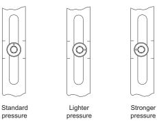
If the sash is clashing with the frame or striker plates, the window must be adjusted by a suitably qualified person.
