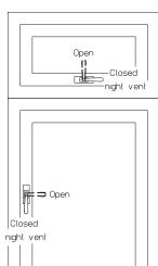
Push button on handle (if applicable) rotate handle 90 degrees and push window open.
