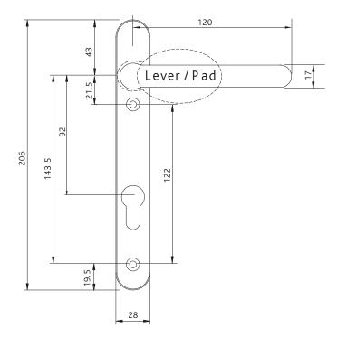
All dimensions are in mm and are nominal. Fab&Fix reserves the right to change specification without notice It is the responsibility of the door manufacturer to ensure that the finished product meets any required safety and performance specification.
